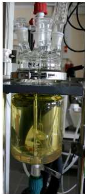
Fig. 7 Laboratory double mantle vessel (2 L)
