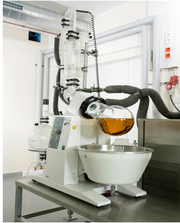
Fig. 8 Rotary evaporator for raw biodiesel drying
