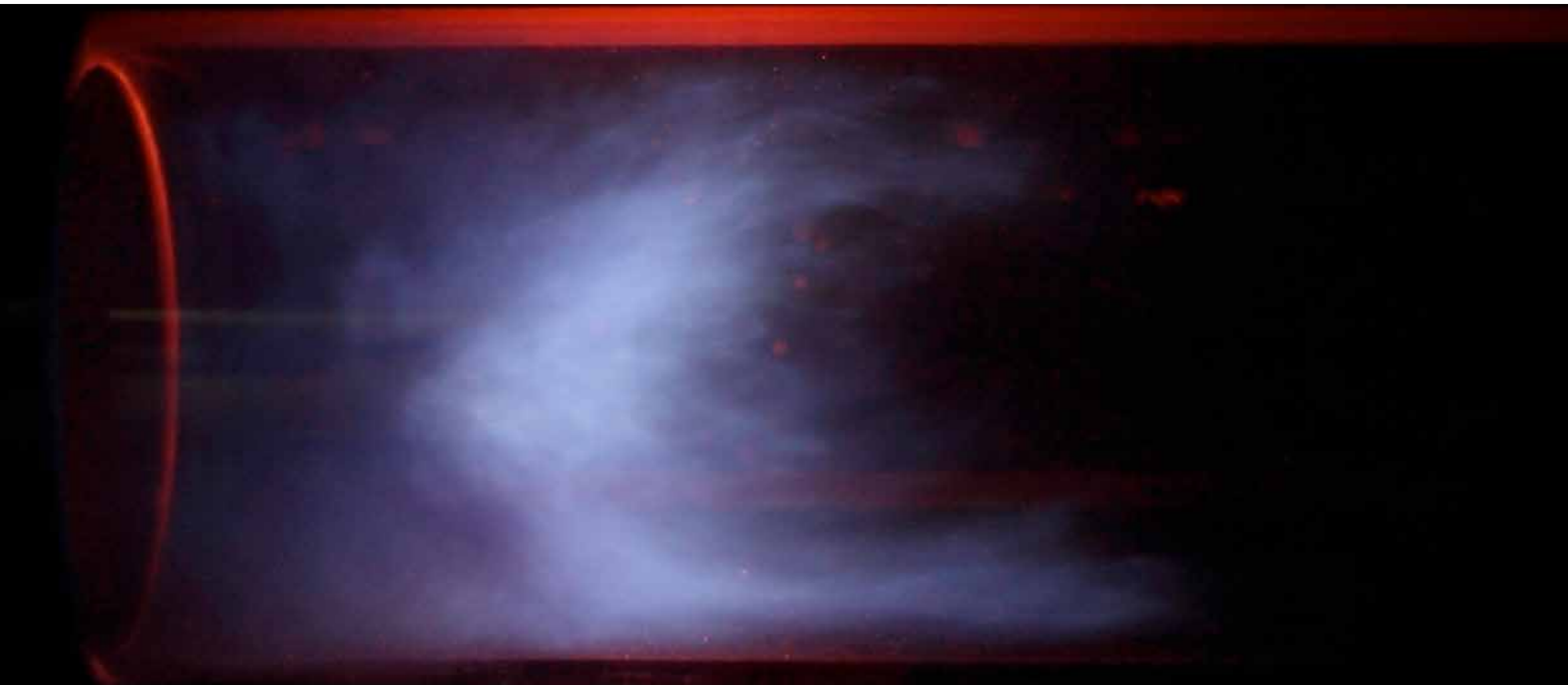
Flammenbild des Brenners auf Basis der Lean-Premixed-Prevaporized-Combustion (LPP). Flame pattern of the burner based on lean premixed prevaporised combustion (LPP). (Photo: OWI)
