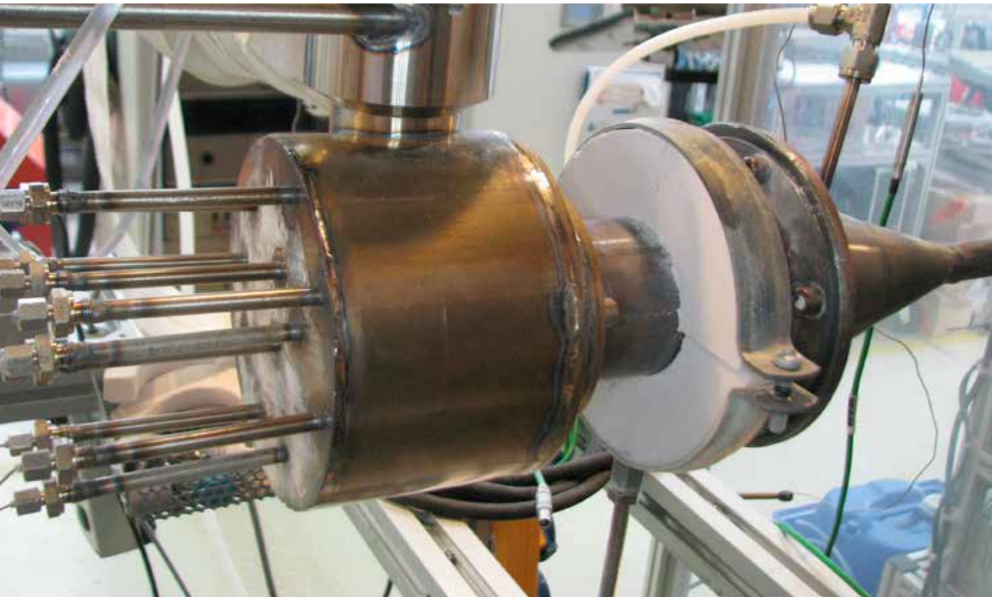
Labormuster des Kalte-Flammen-Verdampfers. Laboratory model of the Cool Flame evaporator. (Photo: OWI)
